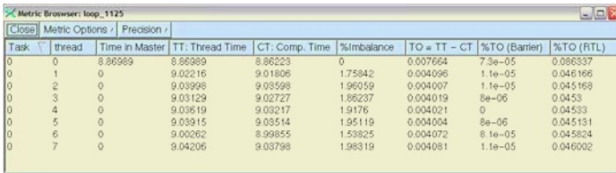
Fig. 4. Detailed view of Loop 1125, modified to use dynamic scheduling
