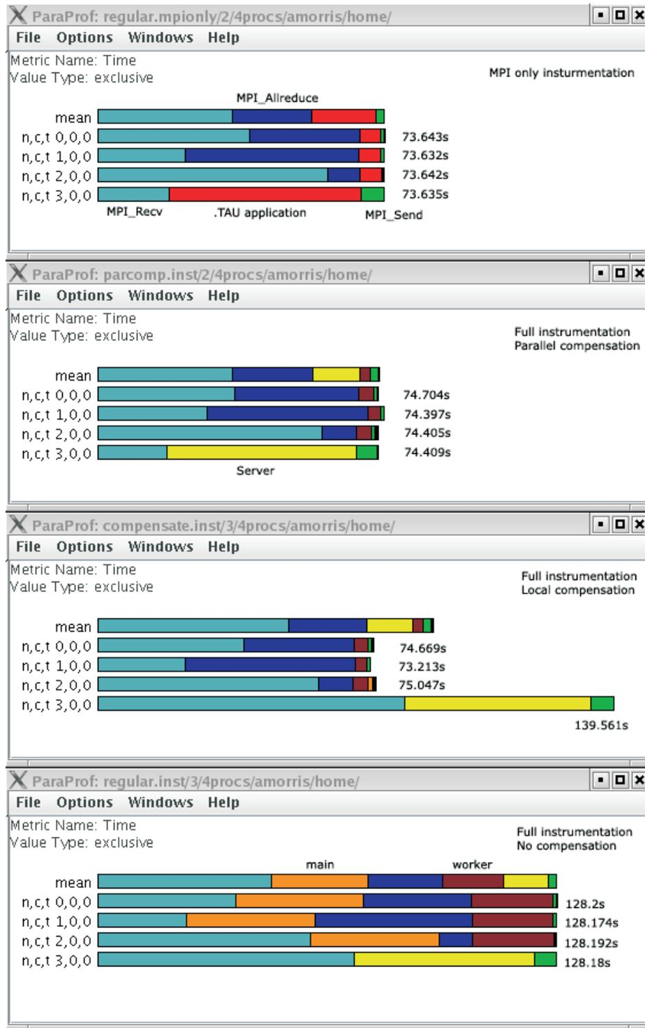
Fig. 13 Parallel overhead compensation in TAU.
