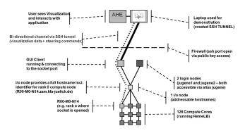
Figure 5. Setup on the BlueGene/P in Jülich to enable computational steering in DEISA.
