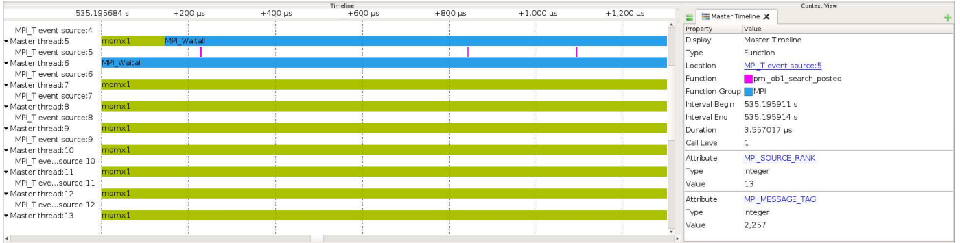
Figure 5: Zoomed timeline of an execution of Zeus-MP/2 on 24 processes. Solid blue lines of the Master thread shows execution of an MPI_Waitall ; Magenta blocks on the location stream below show searches in the posted message queue.
