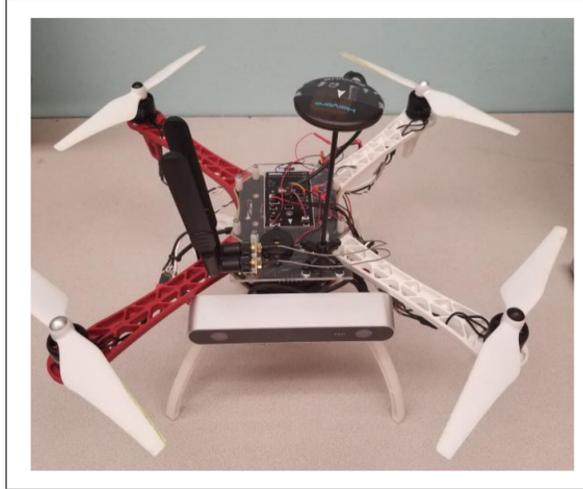
Figure 2: Jetson TX2 board attached on our DJI Flame Wheel drone.
