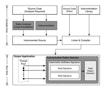
Figure 1. Architecture of the proposed method. Highlighted sections shows the extended modules in DiscoPoP.
