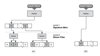
Figure 3. Proposed signature memory architecture. (a) Read signature uses two-level approach, (b) Write signature uses regular signature memory.
