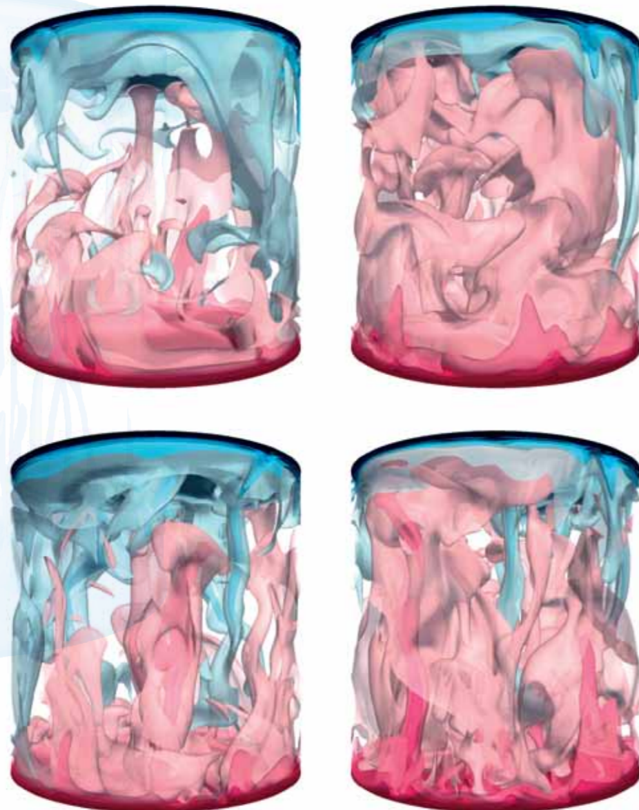
Figure 3: Instantaneous temperature isosurfaces of water ( Pr = 4.38 , Ra = 10^8 , magenta indicates the warm, cyan the cold fluid), shown are the non-rotating OB (upper left) and NOB case (upper right), as well as a moderately rotating OB (lower left) and NOB case (lower right).
