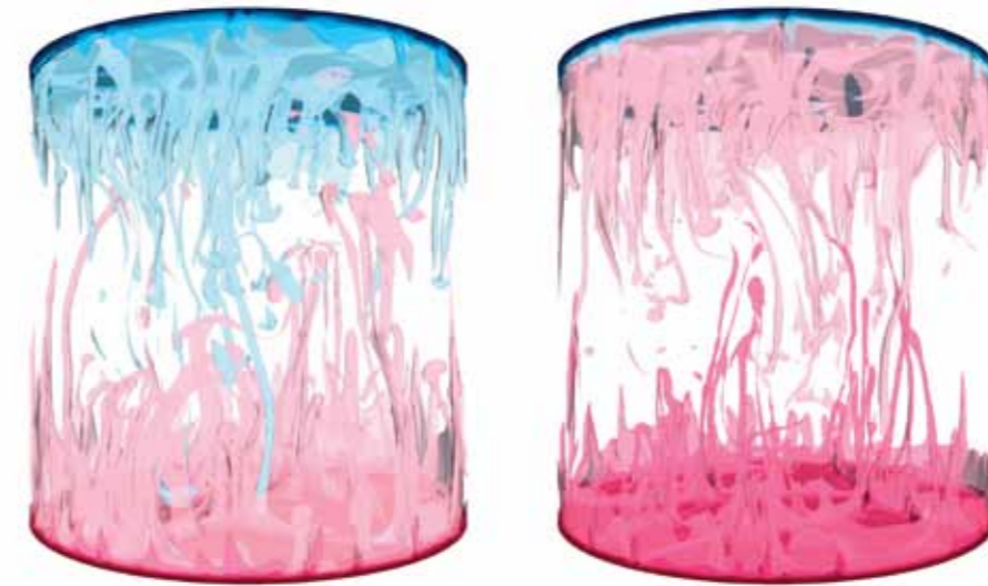
Figure 4: Instantaneous temperature isosurfaces of glycerol ( Pr = 2547.9 , Ra = 10^9 ) under OB (left) and the NOB conditions (right).
