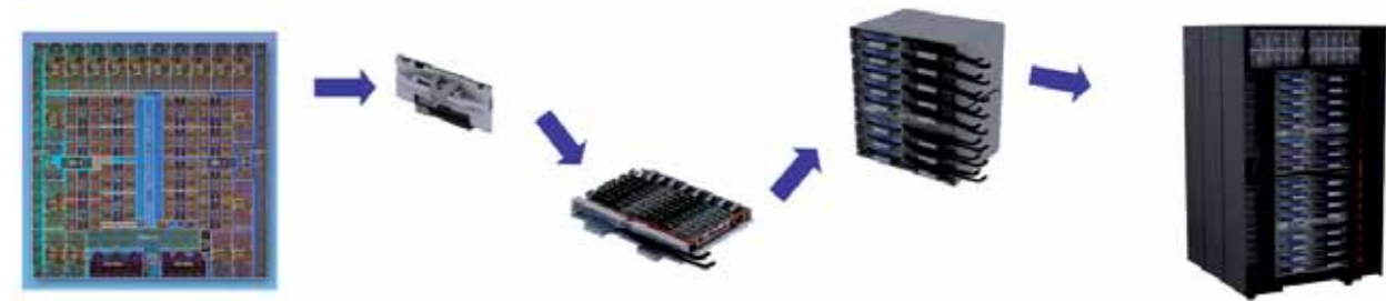
Figure 3: A Blue Gene/Q processor (left) is mounted to a heat spreader. A node-card can host 32 nodes. With 16 node-cards per midplane and two midplanes per rack the total number of nodes per rack (right) is 1,024.
