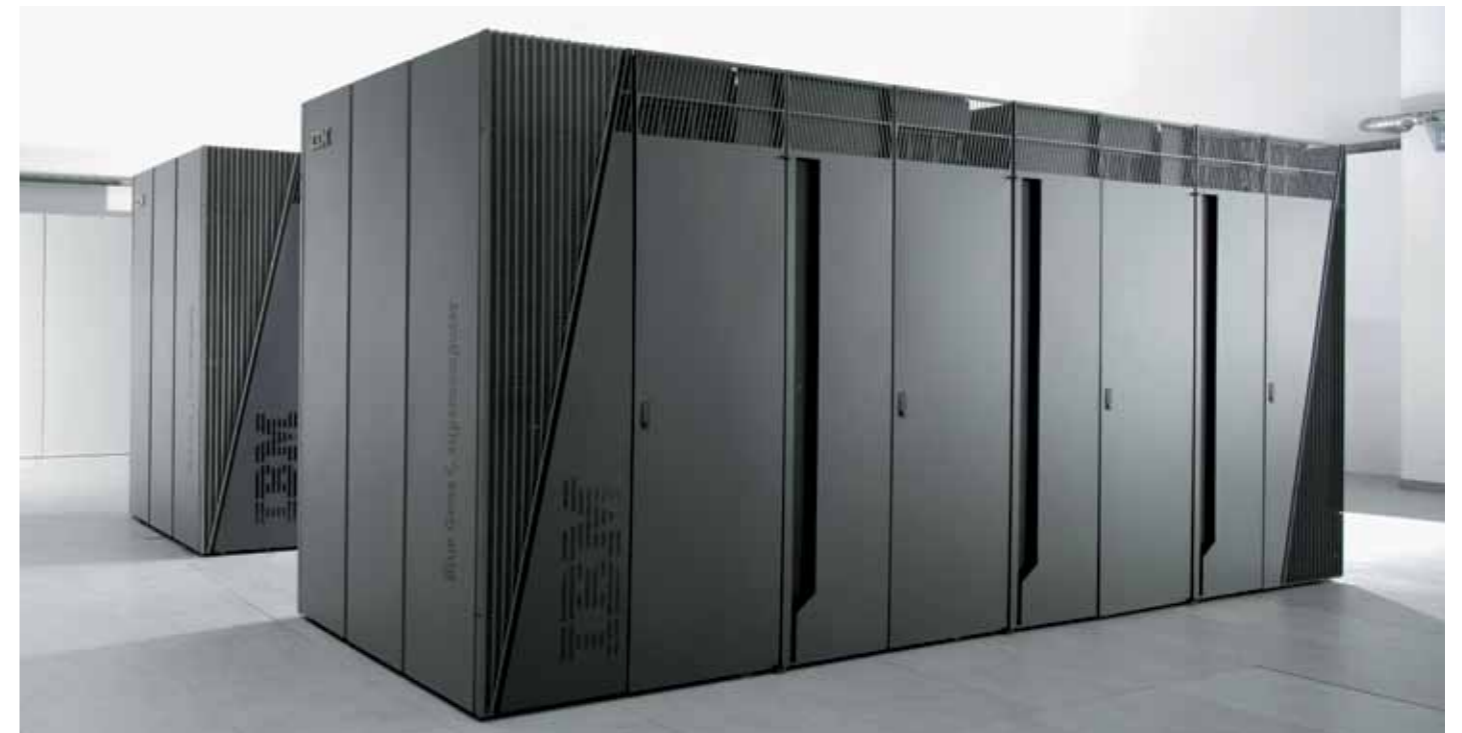
Figure 5: 8-rack JUQUEEN at Forschungszentrum Jülich.
