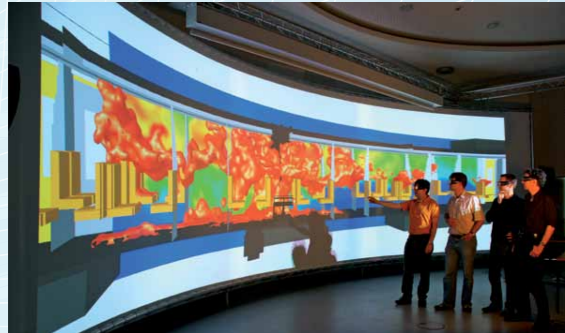
Figure 2: Simulation of fire propagation in a train compartment. Shown is a three dimensional representation of the flame distribution.
