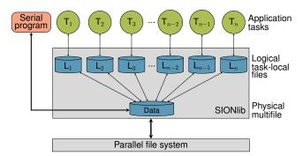
Figure 1: Basic concept of SIONlib: A large number of logical task-local files is mapped onto a single physical file (or a small set of physical files), which is called a multifile. The multifile can be accessed both from a parallel and a serial application.
