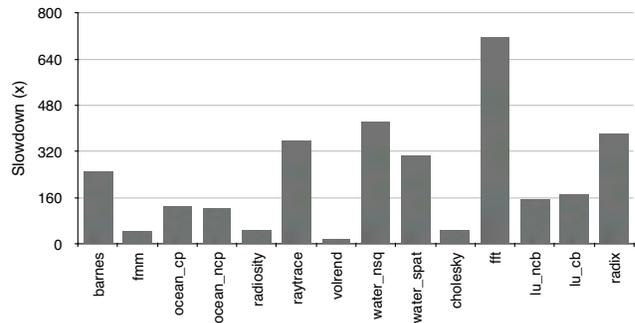
Figure 4. Slowdown of the DiscoPoP on Splash benchmark applications (simdev input size)
