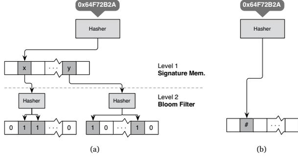
Figure 3. Proposed signature memory architecture. (a) Read signature uses two-level approach, (b) Write signature uses regular signature memory.
