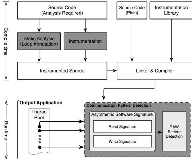
Figure 1. Architecture of the proposed method. Highlighted sections shows the extended modules in DiscoPoP.
