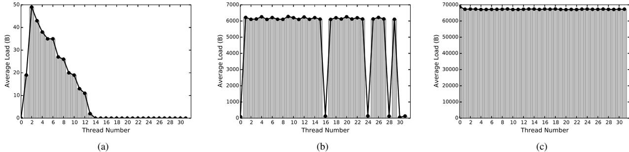
Figure 8. Workload distribution among threads of three hotspots in (a) radix, (b) raytrace and (c) radiosity applications.
