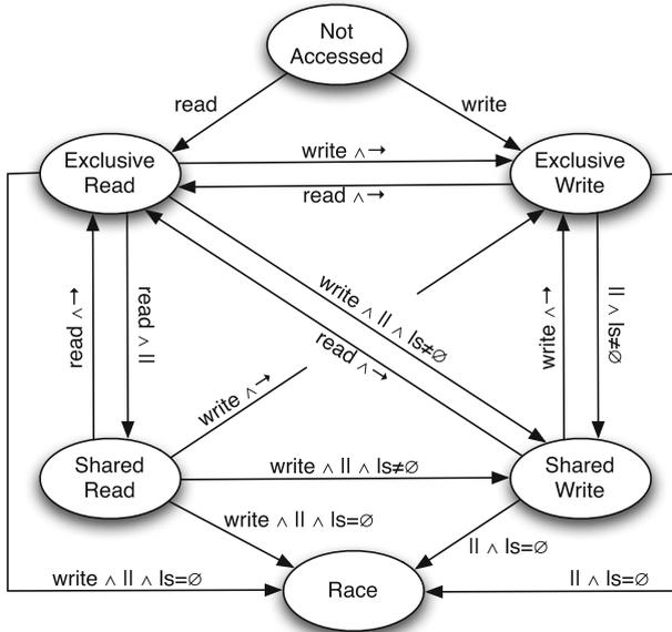
Fig. 11 State machine for correlated sets
