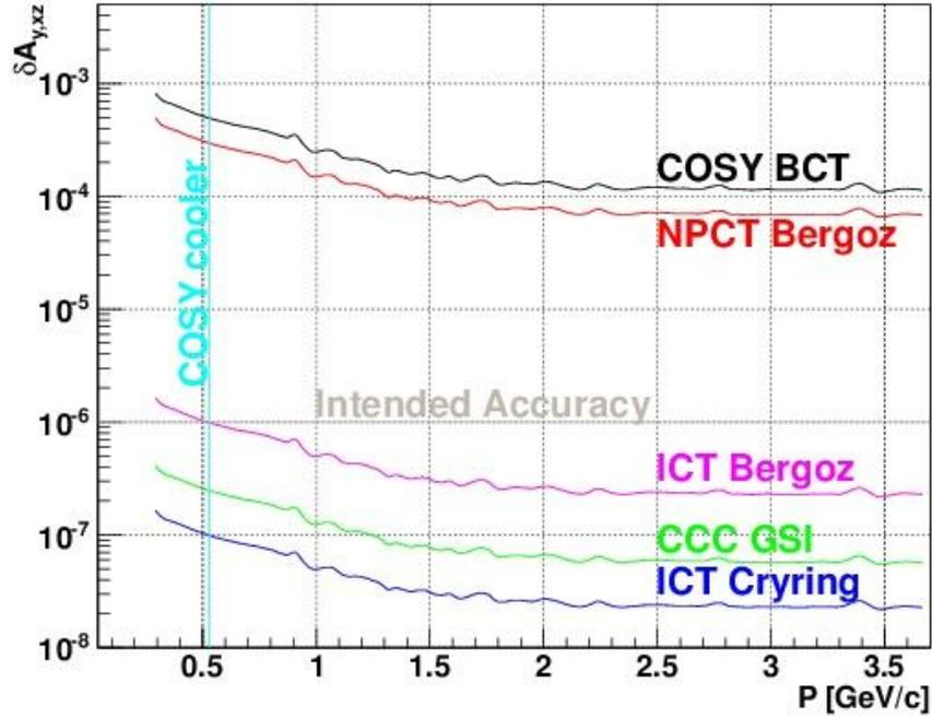
Fig. 6. Different current measuring devices with different errors  $\delta I$  result in different errors  $\delta A_{y,xz}$  for a 30 days run.
