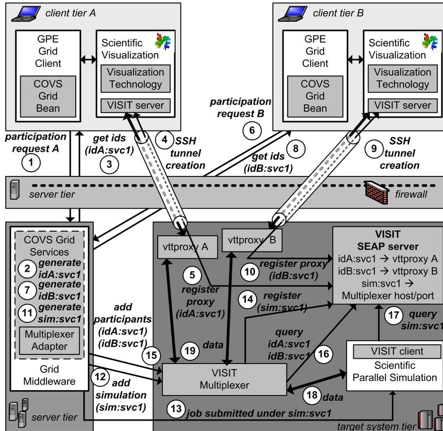
Figure 3. Using the VISIT SEAP server as naming service. Two geographically dispersed participants are dynamically connected using seapservice:seappassword abstractions. SEAP information exchanges are also tunneled via SSH were necessary.
