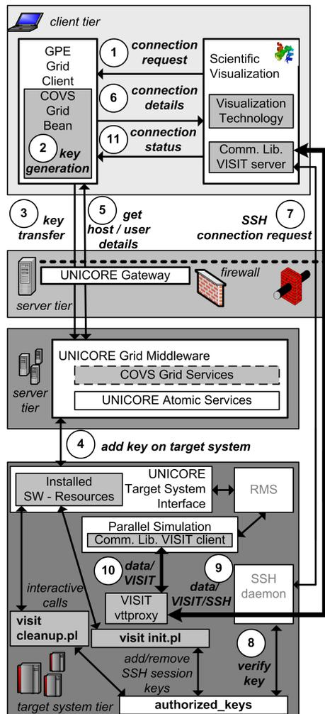
Figure 2. Using interactive calls for the establishment of SSH connections.
