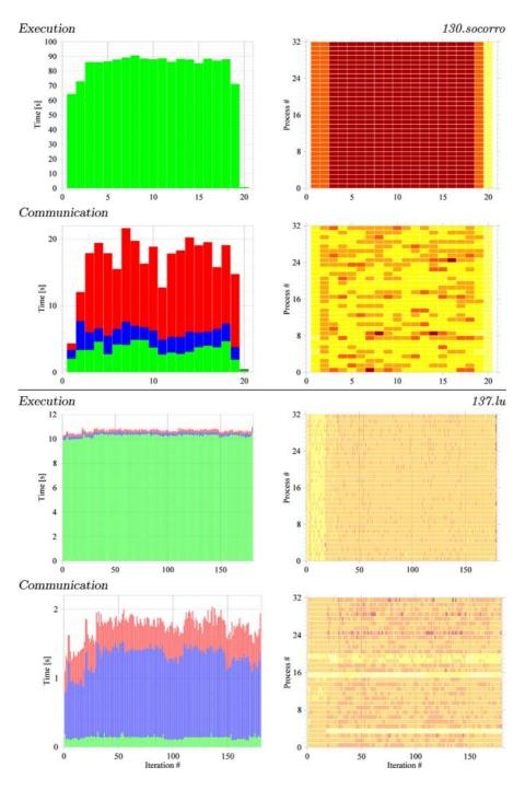
Fig. 5. SPEC MPIm2007 130.socorro and 137.lu iteration time metrics
