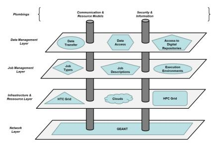
Fig. 1 Interoperablity requirements within four different layers, while two (often behind the scenes realized) plumbings are orthogonal to them because they significantly affect every layer.
