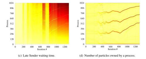
Figure 3. Gradual development of a performance problem along 1,300 timesteps of PEPC on 1,024 processors.
